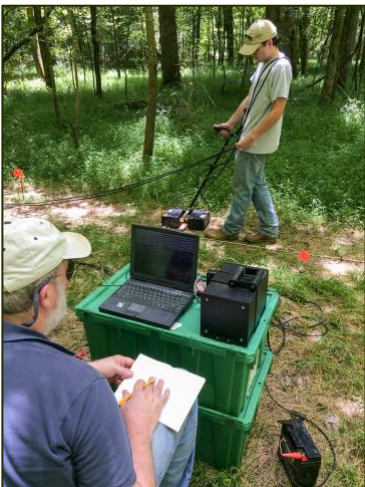
Dr. Ferguson and Ben Thomas '16 use ground penetrating radar to detect what lies below the surface of the land.
